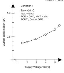
(3-2) Current consumption when non-accessed (ii) when FOUT=32.768 kHz
